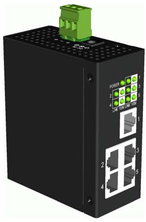
The switch provides five 10/100Mbps copper ports for connections to Ethernet and Fast Ethernet devices. With the featured auto-negotiation function, the switch can detect and configure the connection speed and duplex automatically. The switch also provides auto MDI/MDI-X function, which can detect the connected cable and switch the transmission wire pair and receiving pair automatically. This auto-crossover function can simplify the type of network cables used.
