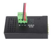
Note: When using terminal block connectors, put a cap on the DC jack.
